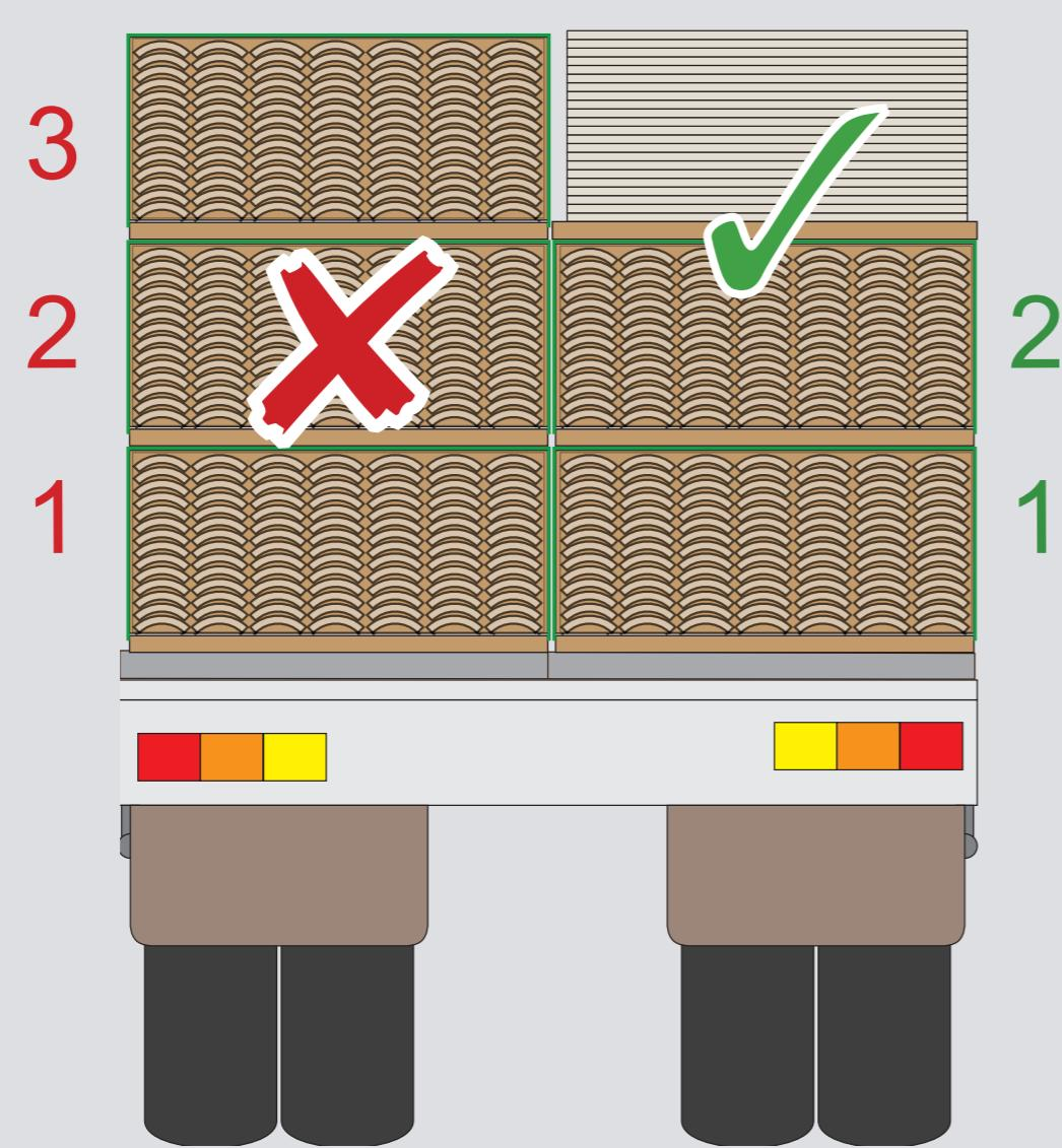
Stack cornice packs on top of sheet packs
