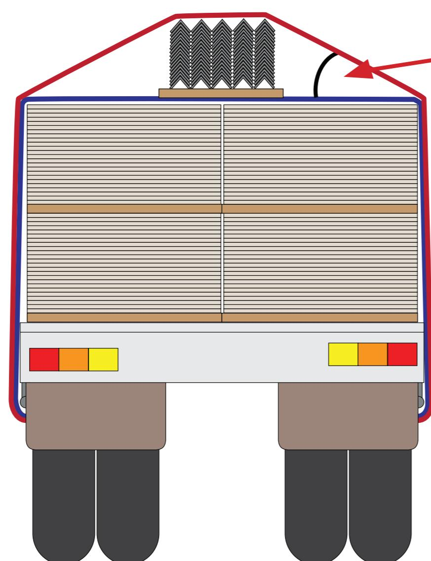
Angle for determining restraint lashings for steel packs
